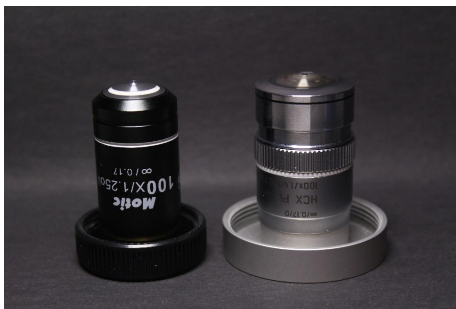
Figure S7. Photograph of the two microscope objective lenses Motic EC PL 100 \times /1.25 (left) and Leica HCX PL APO 100 \times /1.4–0.7 Oil CS (right).
