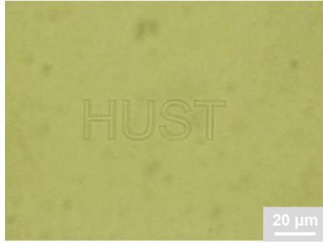
Figure S4. The optical image of the FLDW results on the flexible substrate (PI).
