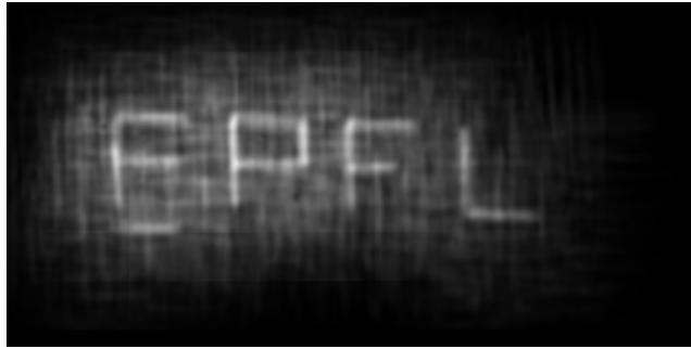
Fig. S15 Last frame of the video. It shows the final NIR dose distribution of the printing.
