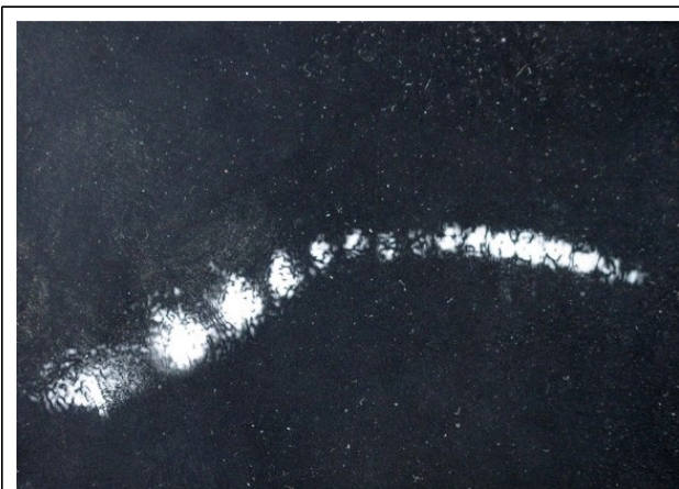
Fig. 1 A reconstruction of a hologram recorded of the object-beam spot seen reflected between two parallel mirrors so that each image has an increased path length of 10 cm 5 . Adapted from Ref. 5 with permission from Optica Publishing Group.
