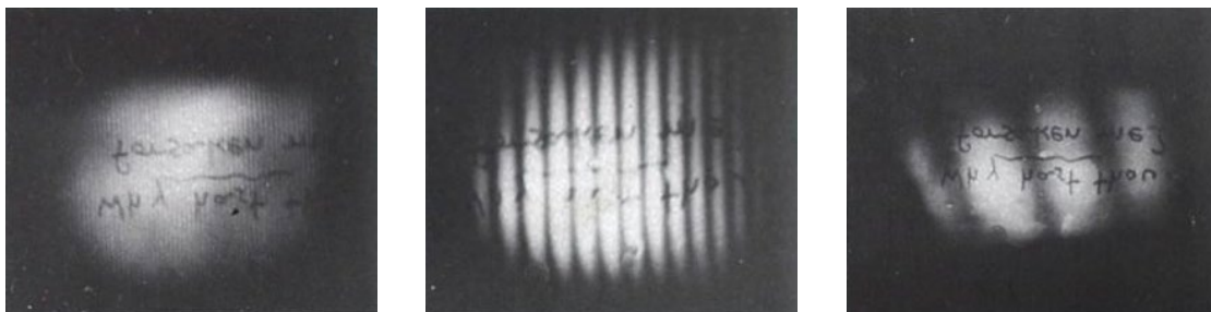
Fig. 3 Reconstructions from double-exposure holograms where the object was given small rotations between exposures. In the first figure, the fringes are too fine to resolve, but were quite visible in the original.
