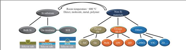
Fig. 1 Schematic overview of heterogeneous Si photonics and its developing branches. Inset: cross-sectional cartoon of three basic waveguides enabled by heterogeneous integration.
