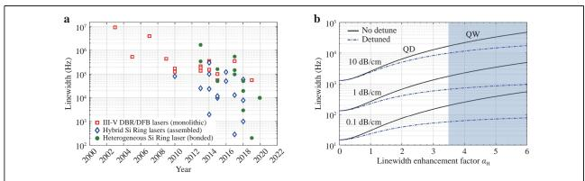
Fig. 7 a Historical progress of Lorentzian linewidth reduction in diode lasers over the past 20 years<sup>92</sup>, and **b** calculated Lorentzian linewidth at 1 310 nm as a function of the  $\alpha_H$  factor for different passive waveguide loss values<sup>111</sup>.
