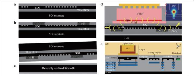
Fig. 11 a-d Schematic fabrication flow to form a special back-side SOI structure with a heterogeneous DFB laser on the top. Inset: simulated TE lasing mode<sup>169</sup>. e Schematic of a similar heterogeneous laser with several monolithic Si photonic components and metal stacks comprising several layers<sup>170,171</sup>.
