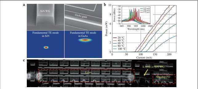
Fig. 4 a SEM images of fabricated SiNx and GaAs waveguides and their respective fundamental TE mode profiles, **b** temperature-dependent LIVs and room-temperature spectra at different injection currents, and **c** top-view microscopic image showing the integrated laser, passive SiN<sub>x</sub> waveguide, and PD $^{\neg}$ .
