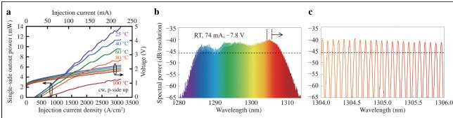
Fig. 8 a Temperature-dependent LIV characteristic of a heterogeneous QD FP laser, **b** Optical spectrum of the comb laser. **b** optical spectrum of the comb laser over the full wavelength range, **c** enlargement of the range indicated in **b** to show individual lasing modes. The dashed line is drawn at –6 dB from the peak comb line [31].
