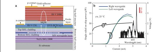
Fig. 3 a Cross-sectional schematic of VCSEL with in-plane out-coupling into a SiN<sub>x</sub> waveguide, and **b** device light-current-voltage (LIV) characteristic showing symmetric coupling to the waveguides on the right and left and cw lasing at 856.5 nm<sup>23</sup>.
