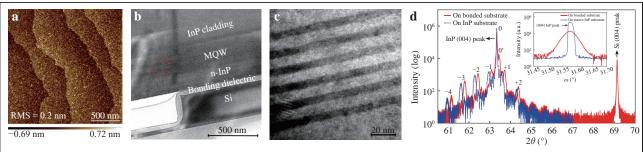
Fig. 13 Images for characterisation of the fabricated device. a AFM, b TEM, c enlargement of the area enclosed within the red square in b, and d high-resolution X-ray ω-2θ measurement of the epitaxy. Inset: high-resolution omega scans of the InP (004) peak<sup>203</sup>.
