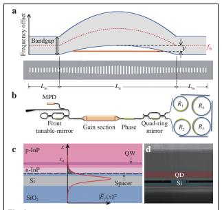
**Fig. 6** a Schematic photonic band gap structure and top-view of the high-Q grating-based laser cavity geometry in <sup>50</sup> and **c** its heterogeneous cross-sectional schematic with lasing mode profile, **b** schematic of a MQW-based heterogeneous extended cavity laser structure <sup>52</sup>, and **d** SEM cross-sectional image of a similar QD-based extended cavity laser <sup>105</sup>.
